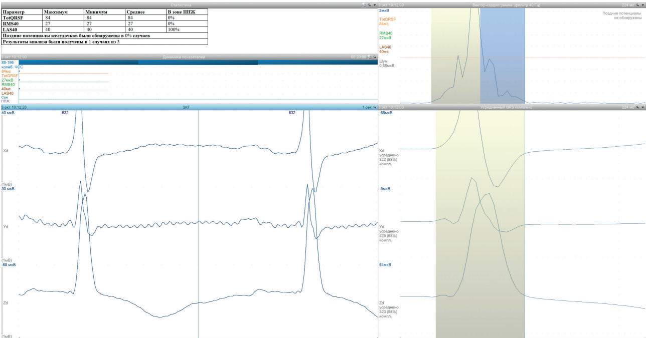
Figure 2. Application of the ventricular late potential detection option to identify signs of anterograde conduction via the accessory pathway (AP) in patient G. The Frank leads are shown (bottom left), along with the result of coherent averaging of QRS complexes (225 to 323 complexes) until the required noise level was achieved (bottom right), and the filtered QRS complex (top right). Explanations in the text.
